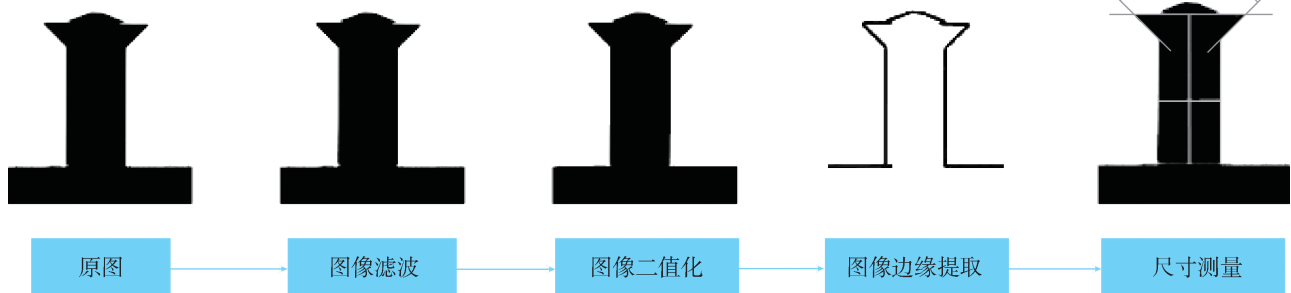
图3 铆钉尺寸自动测量算法流程 Fig.3 Process of rivet automatic detection algorithm
